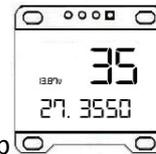
To stop the radio from scanning just push the channel knob in once and it will stop
