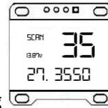
the level you want push the channel knob in and the radio will start scanning you will notice the word SCAN will be on the left hand side above the Voltage readout.
