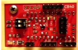
After you have made sure all your wiring is correct and no solder bridges (**Triple check all your work before you apply any power to the radio**), you will need to make sure Switch 2 is on, like you see in [fig 1](#)
